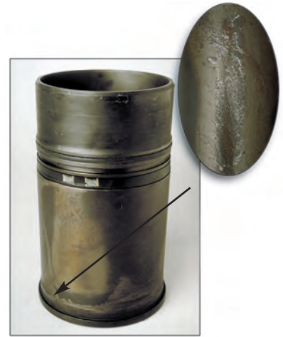
Engine Liner Pitting
