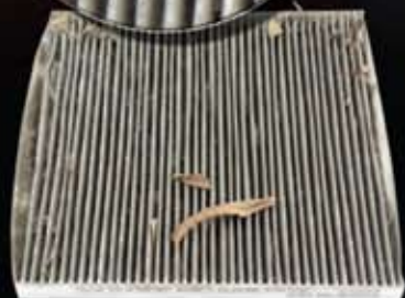
Dirty Cabin Air Filter
